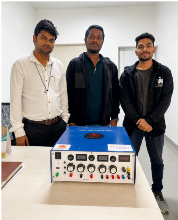
Figure 2. A 3-channel DC power supply built by MSc (Physics, 2024-26) students (Mr. Soham Sahu, Mr. Krushna Chandra Mahali, and Mr. Kruttibasa Danduasi)
